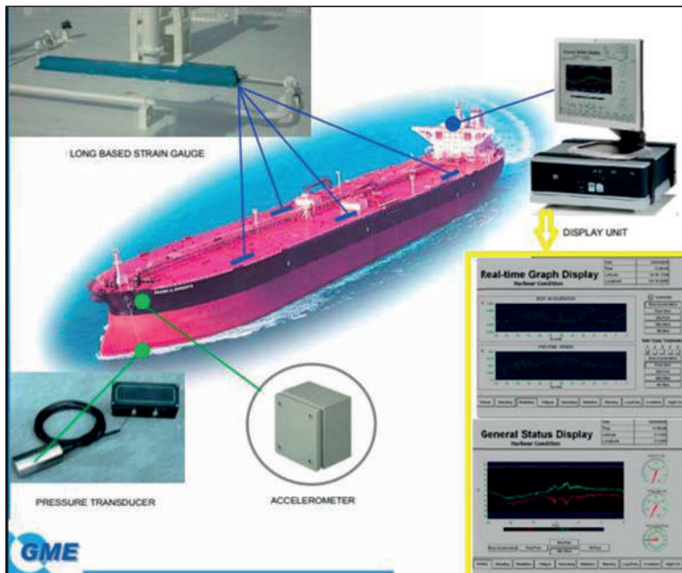
Figure 2 - Typical hull stress monitoring system (with electric sensors) [9]
